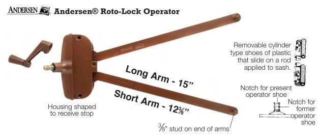
Andersen® Roto-Lock operator comes complete with handle, rods, brackets and screws.
