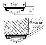
3/8" to 1/2" maximum clearance required between door and threshold
