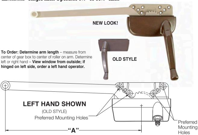
Comes in right hand or left hand. Available in  $9\frac{1}{2}$ " or  $13\frac{1}{2}$ " arm length. The 11" version has been discontinued. Order the  $9\frac{1}{2}$ " version as a replacement. Shipped complete with No.11454 crank handle and screws.
