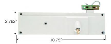
The Truth® manual skylight operator system is easy to install and is compatible with wood, metal or vinyl framed skylights. The special high gear reduction provides the low torque needed to lift a sash weight of 140 lbs. with minimum effort. The steel chain is detachable at the sash for easy maintenance.
